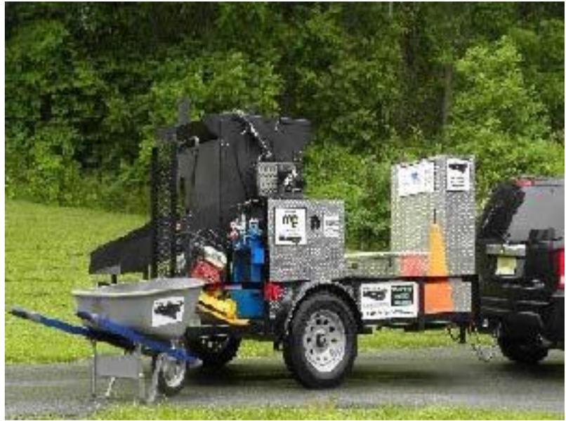
**Simply place a 35lb biodegradable premix bag of PelletPATCH into the Asphalt Patch Master Hopper for approximately 10 minutes**
