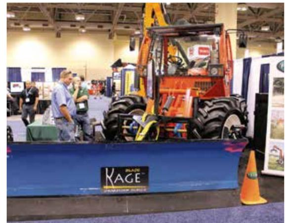
The Fecon booth featured a 12-foot (3.66 metres) Kage blade Snow-storm Series. The blade features a Tri-Formed Box that encloses the back of the moldboard to eliminate torque and strain that can otherwise fatigue the entire structure. Baked on powder coat and primer at 400+ degrees safeguards all of the steel components.
