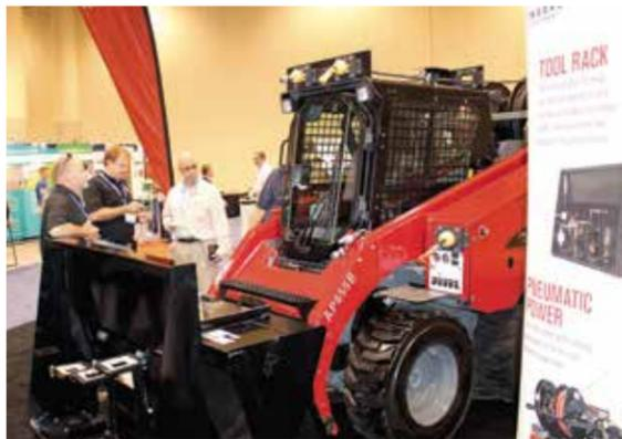
The patent pending all-in-one AMP (Auxiliary Mobile Power) skid steer provides capabilities needed to deliver extreme jobsite performance. A self-contained power source and tool rack allows you to tackle any task efficiently and effectively. This multi-functional unit serves the rugged demands of any jobsite by allowing operators to run an arsenal of tools up to 30.5 metres (100 feet) away. It also has an integral 8.5 kW power source in addition to a fully functioning skid steer loader.
